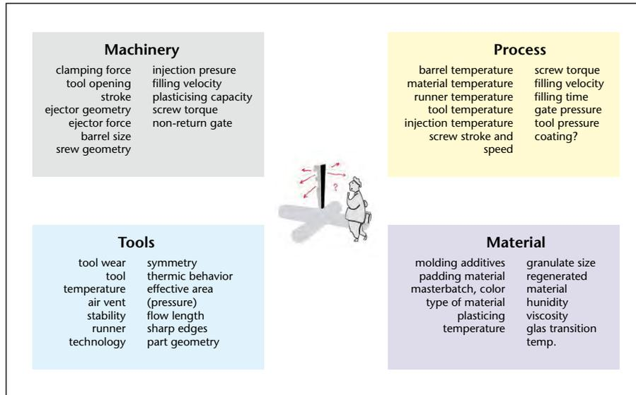
FIGURE 8: Parameters for Injection Molding.
