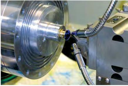
FIGURE 4: MOORE Nanotech 250UPL diamond turning a freeform lens.
