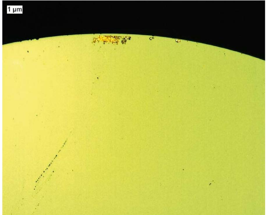
FIGURE 5: Worn out diamond tool tip.
