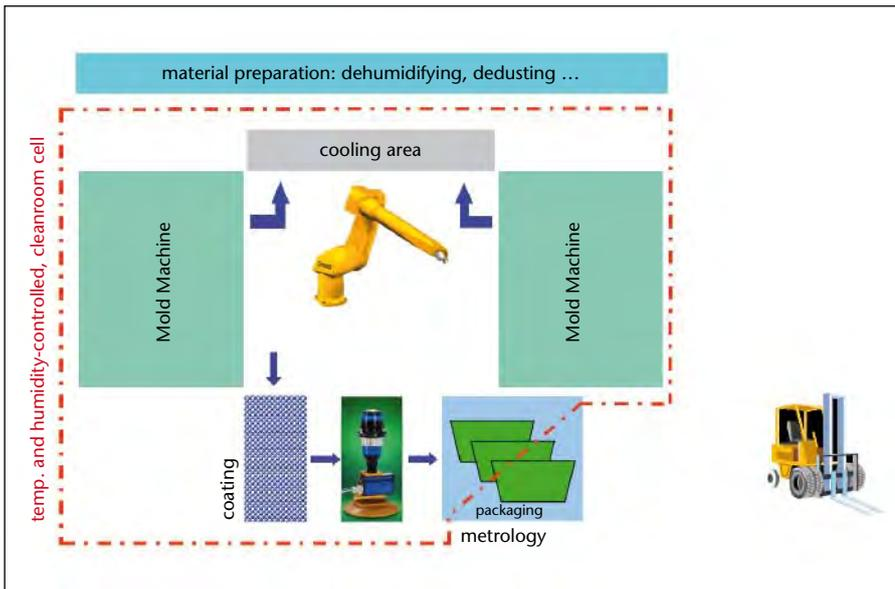
FIGURE 7: Manufacturing Cell (schematic).
