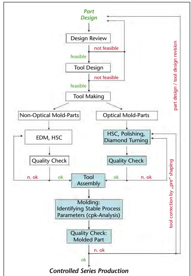
FIGURE 2: From Design to part: High Precision injection molding starts with parts design and ends with the molded part.
